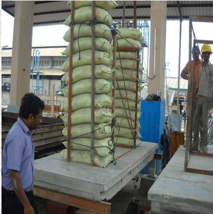
Flexural Test for Sustained Load
