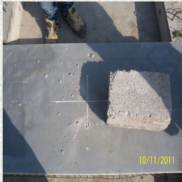
Surface after impact (completely intact after 3 drops)
