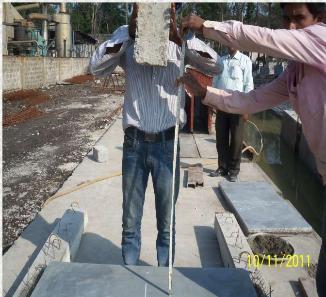
Load of 15 kg being dropped
