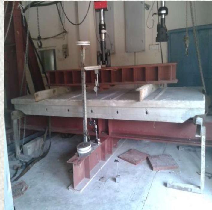
Full Performance Flexural test on MTS, IIT, Hyderabad
